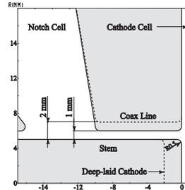
Figure 2: Initial cathode insert geometry [3, 4, 5].
