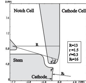
Figure 3: Upgraded geometry of the cathode insert.
