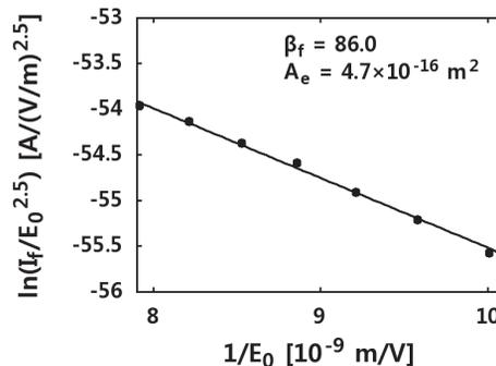
Figure 2: Dark current as a function of maximum surface electric field. The solid line represents a linear fit.
