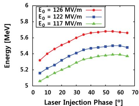
Figure 4: Measured beam energy vs. laser injection phase.
