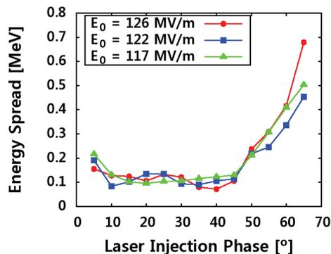
Figure 5: Measured beam energy spread vs. laser injection phase.
