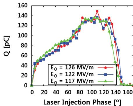
Figure 3: Measured bunch charge vs. laser injection phase.
