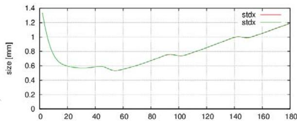
Figure 5: Beam size in the RF gun.
