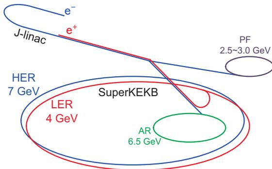
Figure 1: schematic view of KEK accelerator system.
