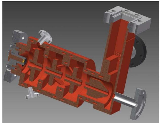
Figure 2: Cut view of DAW type RF gun.
