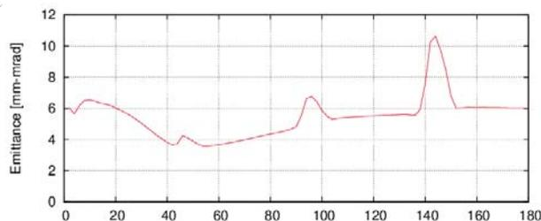
Figure 6: Beam emittance in the RF gun.
