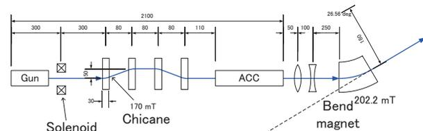
Figure 7: Injection beam line.
