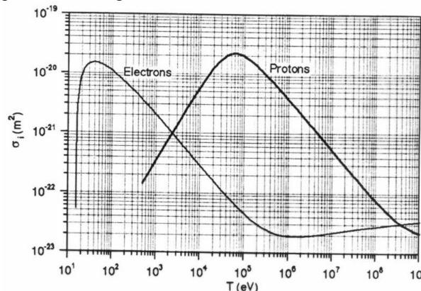
Figure 1: Cross sections of a hydrogen atom ionization by electron and proton .Cross sections of air components ionization are ~6 time larger.
