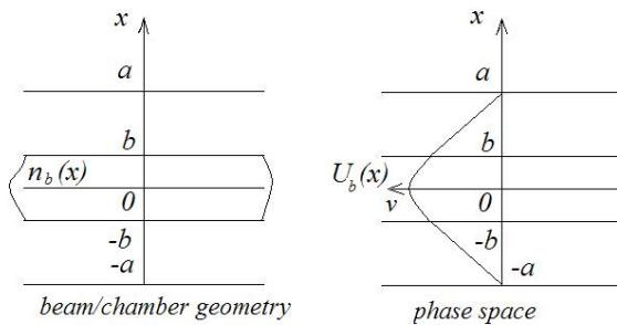
Figure 2: Geometry of one dimension problem( flat beam between two plates) and phase space plane  $x, v$ , and beam potential distribution.
