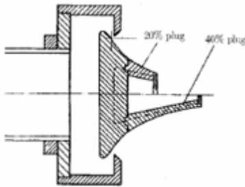
Figure 4: Example of the plug nozzle with a central body for low divergence jet production.
