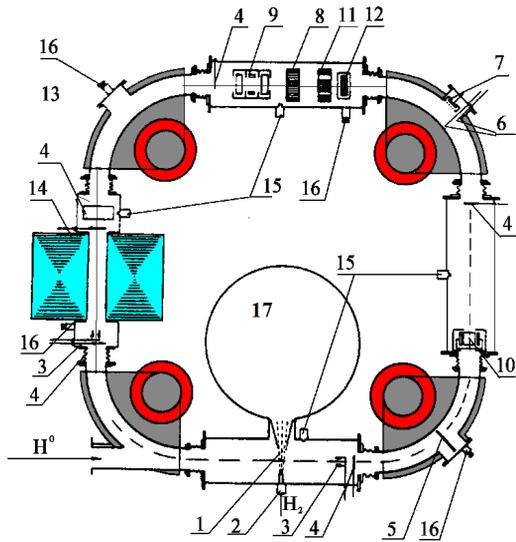
Figure 1: Schematic of storage ring with gas jet stripping target and with diagnostics and control. 1-stripping gas target; 2-pulsed gas valve; 3-Faraday Cup; 4-Quartz screen; 5, 6-moving targets; 7-ion collectors; 8-current monitor; 9-Beam Position Monitor; 10-Quadrupol pick ups; 11-magnetic BPM; 12-beam loss monitor; 13-detector of secondary particles density; 14-inductor core; 15-gas pulses; 16-gas leaks, 17-jet receiver and pumping.
