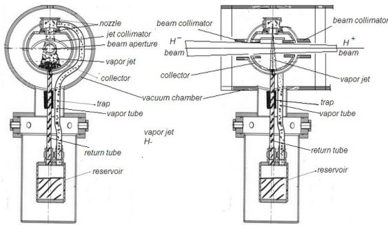
Figure 3: Jet formation with vapour recirculation [14]
