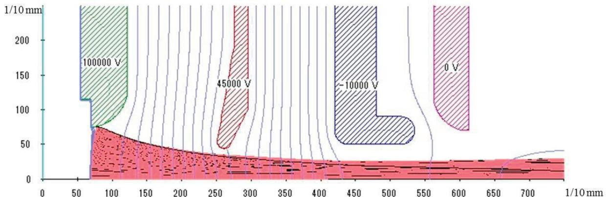
Figure 1: Arrangement of extraction electrodes.
