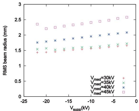
Figure 5: Beam radius change for the voltages applied to the medium electrode and the suppresser electrode.
