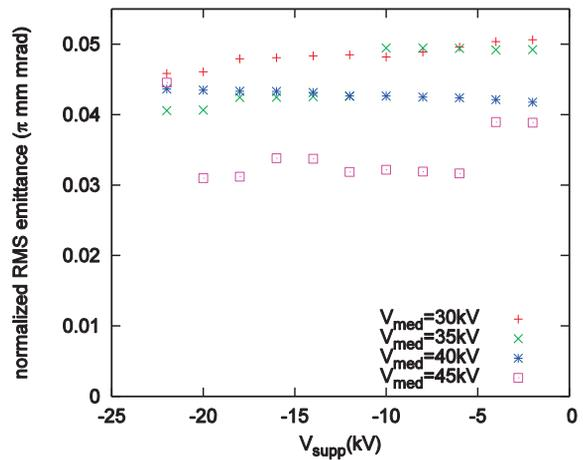
Figure 4: Emittance change for the voltages applied to the medium electrode and the suppresser electrode.
