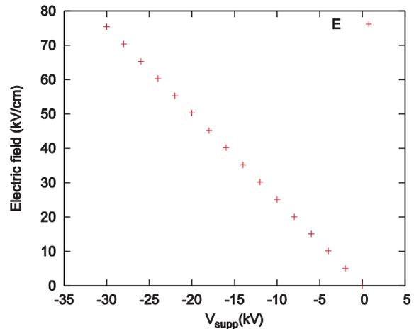
Figure 3: Electric field between the suppresser electrode and the ground electrode.
