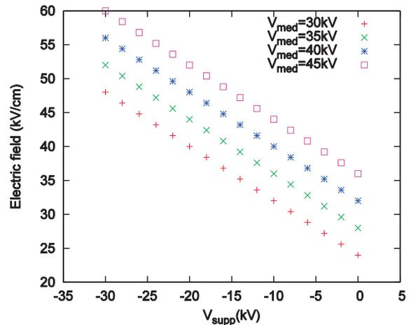
Figure 2: Electric field between the medium electrode and the suppresser electrode.
