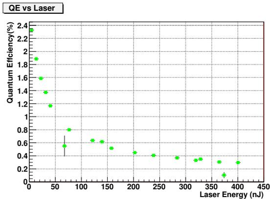
Figure 3: Quantum efficiency as a function of laser energy per bunch.
