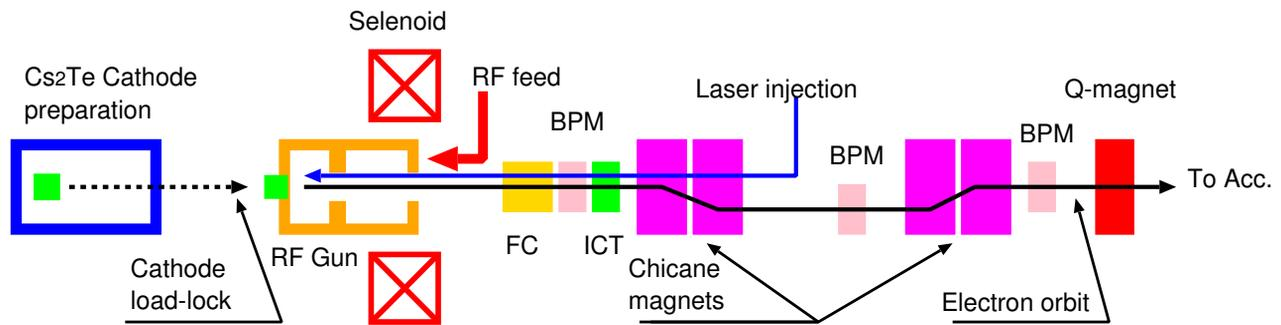
Figure 1: Injector setup for STF beam line. Chicane orbit is designed for laser injection in right angle to cathode surface. Beam current and position are measured by FC (Faraday Cup), ICT (Integrated current Transformer), BPM (Beam Position Monitor). Solenoid and Q-magnet are set for beam focusing and transporting.
