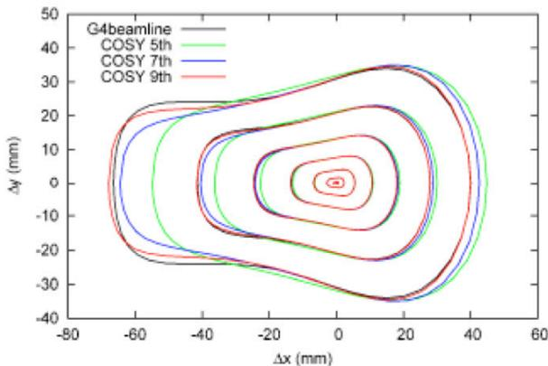
Figure 5: G4beamline simulation is compared to various-order COSY Infinity calculations. Here, beam smear due to spherical aberrations after 2 periods of an epicyclic PIC channel [5].
