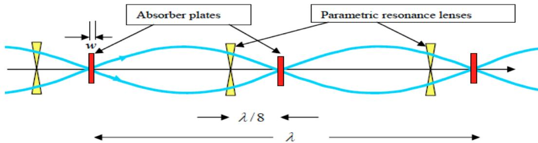
Figure 3: Trajectories (blue) indicate the betatron motion of particles that define the beam envelope in a PIC lattice. Dispersion is low at the absorber wedges (to minimize energy straggling) but not zero (to enable emittance exchange)
