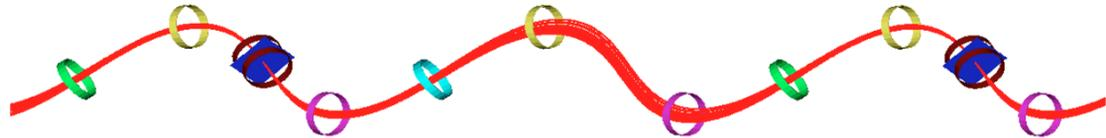
Figure 4: A G4beamline (described below) simulation display of particle trajectories described by the schematic pictured in Figure 3. The absorbers are blue, the horizontal and vertical parametric resonance elements are green and yellow, respectively. The focal points in both transverse planes are at the absorbers.
