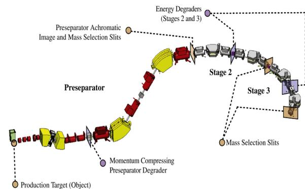
Figure 1. Conceptual design of FRIB fragment separator. A vertical momentum compressing preseparator is followed by two horizontal separator stages. The beam enters from the left. Figure 1: Layout of papers.
