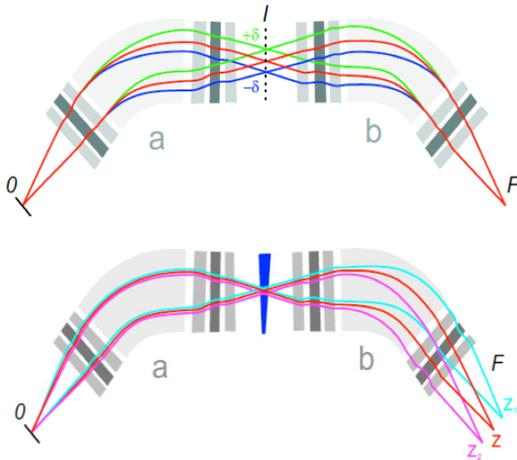
Figure 2: (top) Ion optics of an achromatic magnetic separator. (bottom) Three different isotopes with the same  $m/q$  ratio and the same velocity pass through the first spectrometer stage. A degrader at the intermediate plane slows the beam particles down depending on their nuclear charge. The velocity difference separates the isotopes in the second stage.
