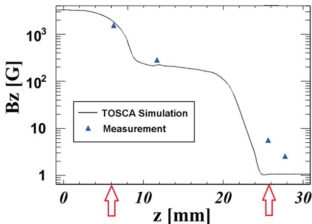
Figure 5: Simulation and measurement comparison of the prototype magnetic plug. Arrows indicate span of the plug.
