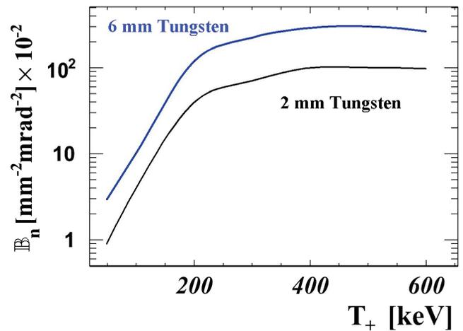
Figure 3: Normalized brightness ( $=\eta_+/\epsilon_x\epsilon_y$ ) of  $e^+$  after the plug with  $T_+ < 600$  keV for 2 and 6 mm tungsten thickness.
