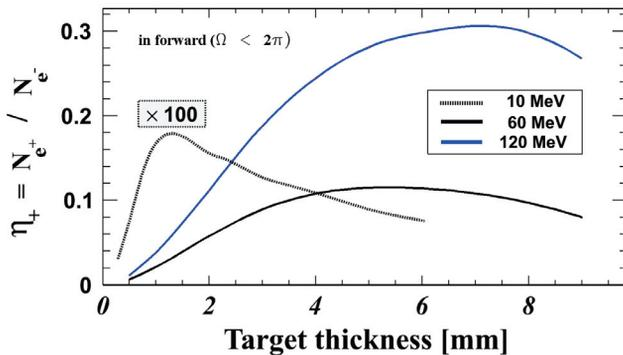
Figure 2:  $\eta_+$  as a function of the W thickness. The 10-MeV curve is multiplied by 100 for convenience.
