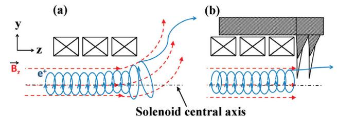
Figure 4: Concept of transport through the solenoid channel (a) without and (b) with the magnetic steel plug. Solid blue lines show  $e^+$  track. Dashed red lines are magnetic field lines. Only the upper half of solenoid is shown.
