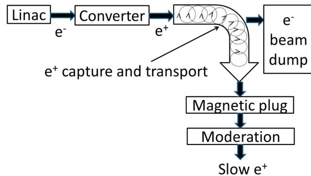
Figure 1: Concept of the low-energy  $e^+$  source.
