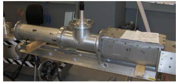
Figure 5: The thyatron housing with HV input.
