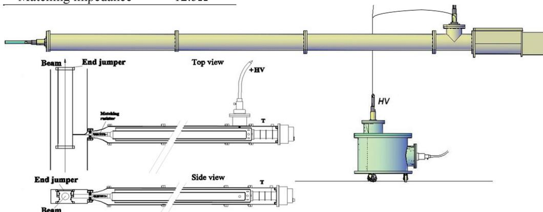
Figure 4: The Blumlein generator prototype. At the left: The Blumlein pulser as a three-coaxial line. Outer diameter of the Al tubing is 7", length of each section  $\sim 1.5$  m. In the final model diameter will be reduced to 4" OD. Inner volume filled with oil. T stands for the thyatron.
