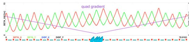
Figure 3a. Increasing quadrupole strength with distance to center of linac and 1<sup>st</sup> whole pass beta functions.
