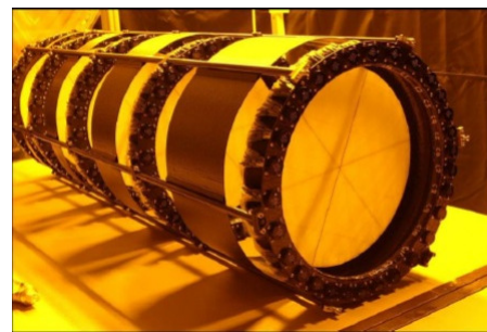
Figure 2: The MICE scintillating-fibre tracker.
