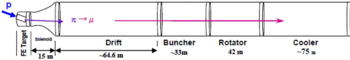
Figure 1: Overview of the IDR neutrino factory front end, consisting of a target solenoid (20 T), a capture solenoid (20 T to 1.5T, 15 m), Drift section (64.6 m), rf Buncher (33 m), an energy-phase Rotator (42 m), and a Cooler (75 m).
