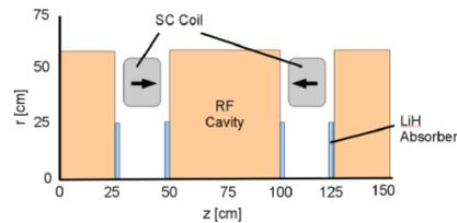
Figure 2: A cooling cell (schematic view).
