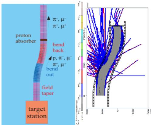
Figure 4: Chicane design concept, and particle loss trajectories from simulation.
