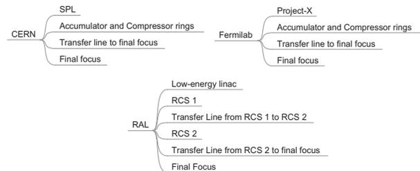
Figure 2: High-level breakdown of the three proton driver options for the IDS-NF.
