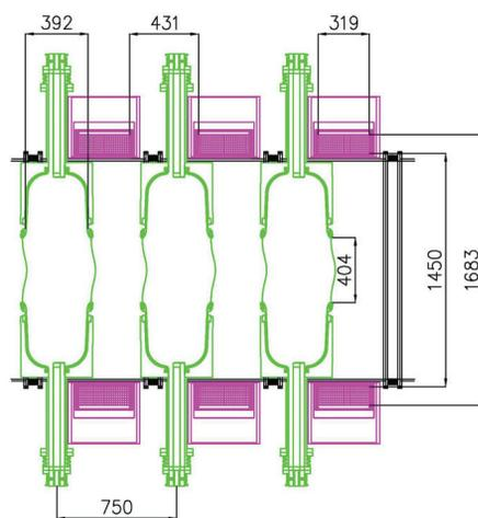
Figure 3: Schematic drawing of the buncher module showing the arrangement of the coils, cavities and RF power input couplers.
