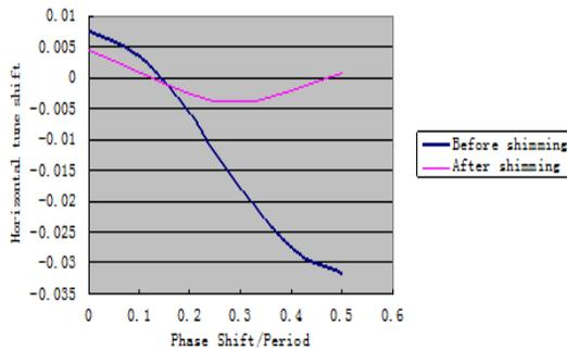
Figure 10: Horizontal tune shift in EPU148 before and after shimming.
