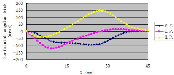
Figure 9: Horizontal angular deflection as a function of the horizontal position in the mid-plane of EPU148 after shimming.
