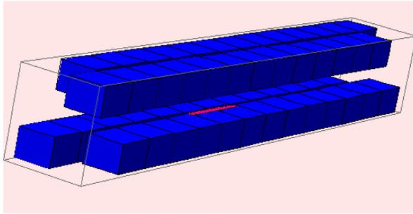
Figure 8: Shim geometry for EPU148 tune shift.
