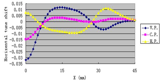
Figure 4: The horizontal tune shift as a function of the horizontal position in the mid-plane of EPU148.
