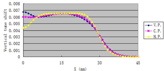
Figure 7: The vertical tune shift as a function of the horizontal position in the mid-plane of EPU58.
