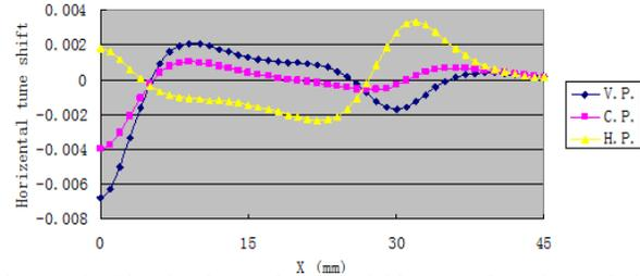
Figure 6: The horizontal tune shift as a function of the horizontal position in the mid-plane of EPU58.
