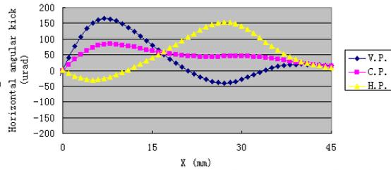
Figure 2: Horizontal angular deflection as a function of the horizontal position in the mid-plane of EPU148.
