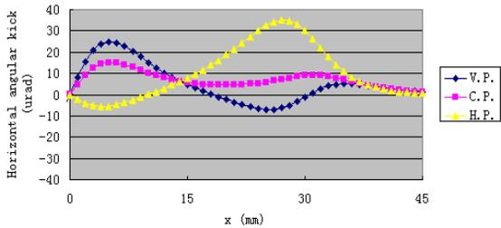
Figure 3: Horizontal angular deflection as a function of the horizontal position in the mid-plane of EPU58.
