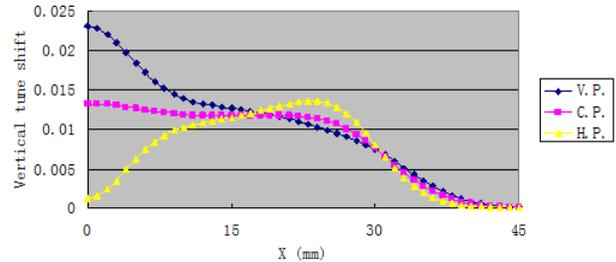
Figure 5: The vertical tune shift as a function of the horizontal position in the mid-plane of EPU148.
