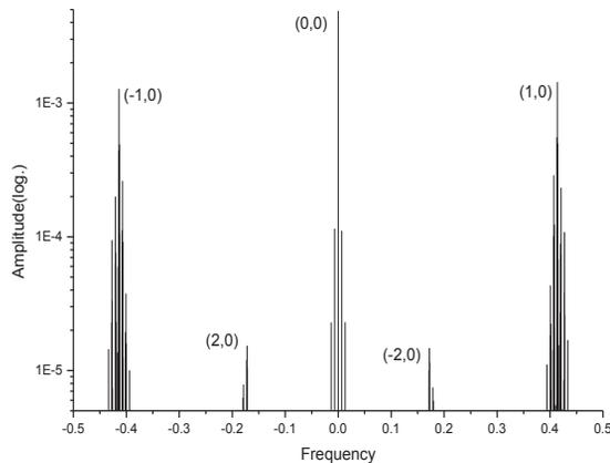
Figure 1: Spectrum of horizontal centroid motion of the beam for the HLS without the effect of radiation damping.
