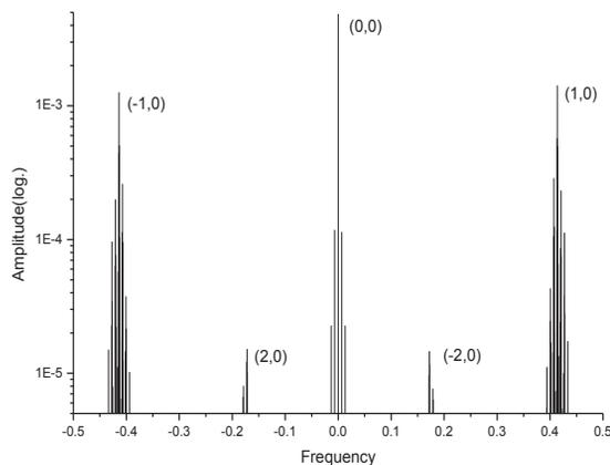
Figure 2: Spectrum of horizontal centroid motion of the beam for the HLS without the effect of radiation damping.
