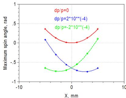
Figure 4: Maximum spin deflection angle after  $10^9$  turns versus  $x$  deviation at  $\Delta p/p=2 \cdot 10^{-4}$ ,  $0$ ,  $-2 \cdot 10^{-4}$ .
