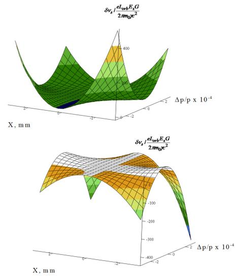
Figure 2: Spin tune aberration dependence on momentum spread and horizontal deviation at different  $k_1, k_2$ .
