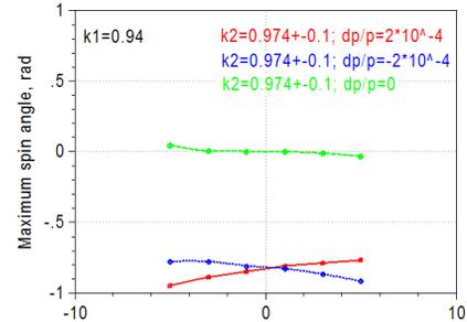
Figure 5: Maximum spin deflection angle after  $10^9$  turns versus  $x$  deviation in mm at  $\Delta p/p=0$  (a) and  $\pm 2 \cdot 10^{-4}$ ,  $0$  (b).
