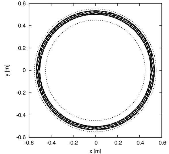
Figure 2: Orbit of a single particle in an azimuthally symmetric toroidal sextupole field. Dashed circles are the intersection of the nominal magnet boundaries with the  $x-y$  plane. The particle was tracked for 1.25 s and traveled 100 m.
