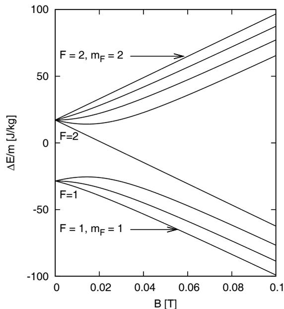
Figure 1: Zeeman splitting of hyperfine ground states of  ${}^7\text{Li}$ . The preferred field-repelled state ( $F=2, m_F=2$ ) and field-seeking state ( $F=1, m_F=1$ ) are indicated by arrows.
