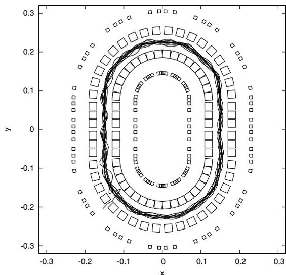
Figure 3: Orbit of a single particle in a discrete-sextupole racetrack ring. The inner rectangles are the intersections of the sextupoles with the  $x - y$  plane and the outer rectangles indicate solenoids. In this case, the particle was lost after 0.4 s and 9 revolutions.
