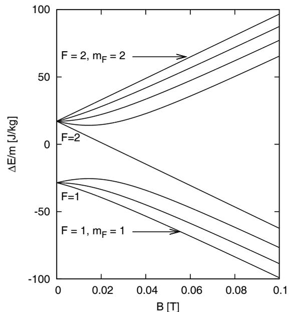
Figure 1: Zeeman splitting of hyperfine ground states of  ${}^7\text{Li}$ . The preferred field-repelled state ( $F=2, m_F=2$ ) and field-seeking state ( $F=1, m_F=1$ ) are indicated by arrows.
