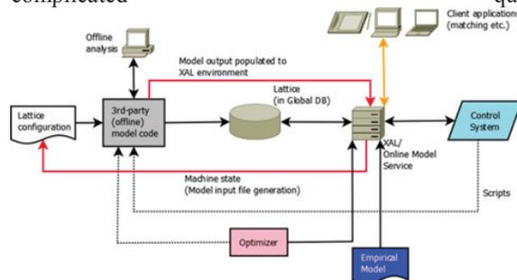
Figure 1: Model Platform schematic diagram.
