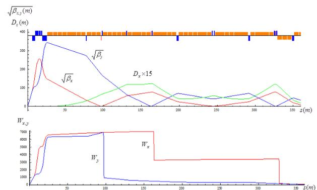
Figure 1: IR and CCS layout and optics functions (top) and chromatic functions (bottom) for  $\beta^* = 5\text{ mm}$ . Orange and blue rectangles represent dipoles and quadrupoles respectively while sextupoles are shown in red. The lattice is symmetric w.r.t. the interaction point at  $s = 0$ .
