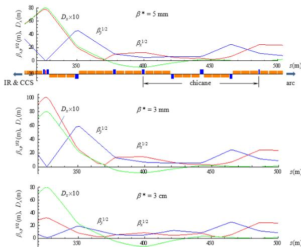
Figure 4: Layout and optics functions in the matching section tuned for indicated values of  $\beta^*$ .
