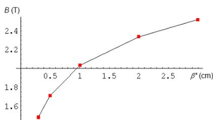
Figure 5: Bending field in chicane vs.  $\beta^*$ .
