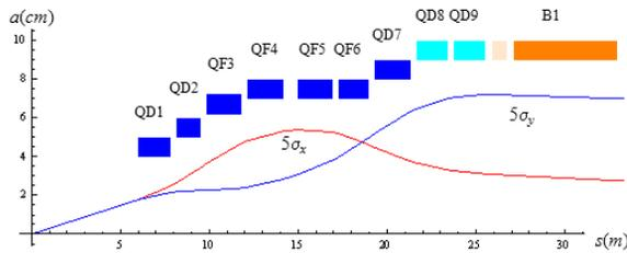
Figure 2: Beam sizes and bore radii of the final focus magnets.
