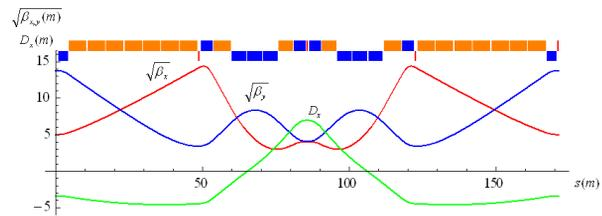
Figure 3: Layout and optics of an arc cell with combined-function magnets.
