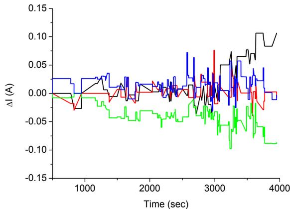
Figure 3: Evolution of non-dispersive skew corrector settings during RWO. The setting of four out of 24 correctors is shown, including unsuccessful steps that were removed before the next step.
