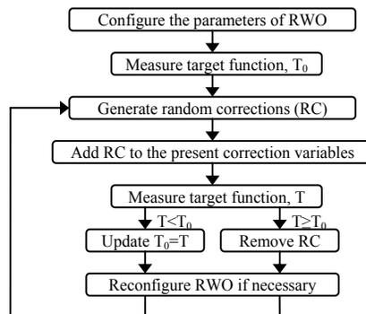
Figure 1: Flowchart of RWO for a minimization of target function  $T$ . RWO is parameterized by a random number distribution (usually Gaussian or uniform), the step size and a set of correction variables.
