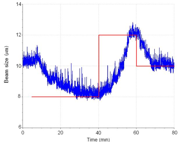
Figure 4: Automatic beam size control with RWO. The blue line shows the measured beam size. The initial beam size was  $\sim 10$   $\mu\text{m}$ . The target beam size was changed as shown by the red line and achieved by an automated RWO. The non-dispersive skew quadrupoles were used as knobs.
