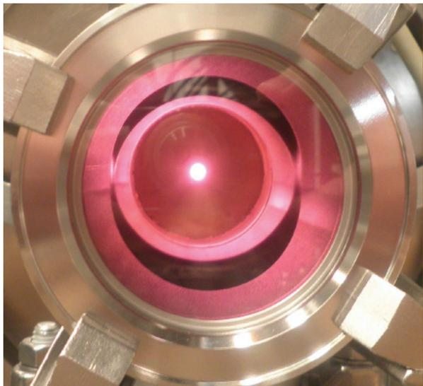
Figure 3: Image of the hydrogen plasma ignited in the chamber viewed through the plasma iris aperture
