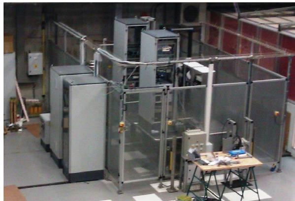
Figure 4: High voltage enclosure for the  $H^+$  source, showing the control and power racks along with the klystron amplifier and RF line.
