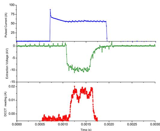
Figure 2: Graph showing the extraction voltage pulse (top), the current pulse into the source (middle) and the extracted beam current measured at the DC current transformer (bottom).
