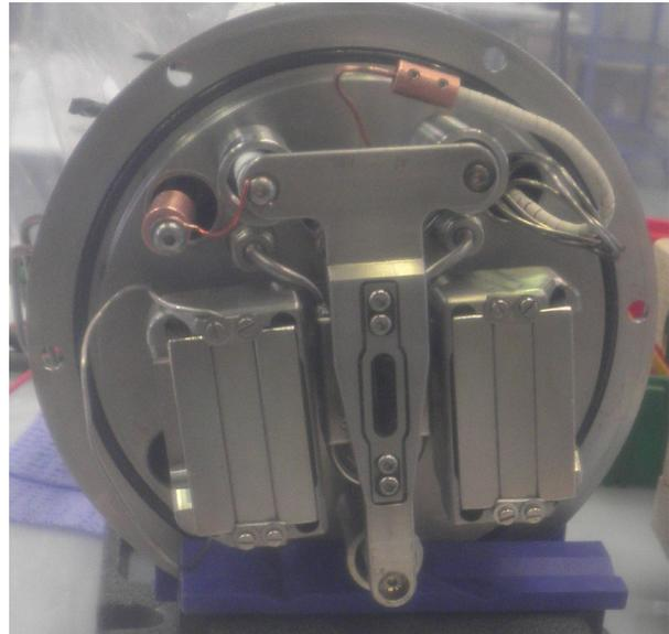
Figure 1: Front view of the modified ISIS source, permanent magnets can be seen on both sides of the extraction electrode.
