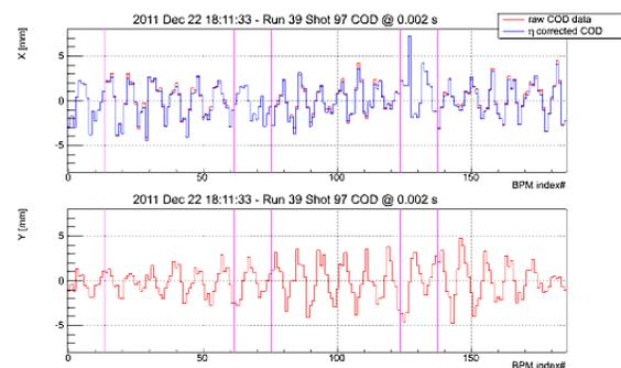
Figure 3: Measured bare COD in horizontal (upper) and vertical (lower) on 12/22/2011 after the Tohoku earthquake and realignment. Horizontal axis is MR BPM index.
