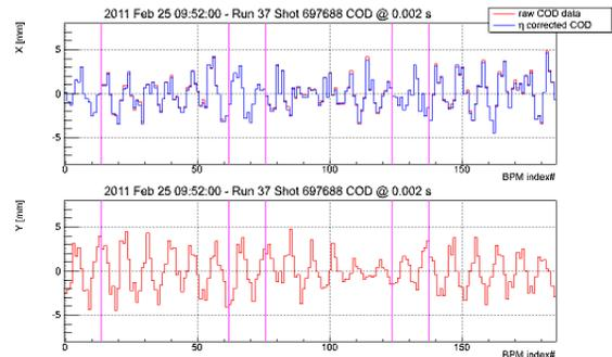
Figure 2: Measured bare COD in horizontal (upper) and vertical (lower) on 02/25/2011 right before the Tohoku earthquake. Horizontal axis is MR BPM index.
