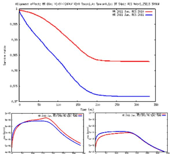
Figure 5: Simulated MR beam dynamics with MR June 2011 alignment in MR 190 kW operation. Horizontal axis is time from injection to end of smoothing acceleration. Red line is for RCS 2010 alignment, blue line is for RCS summer 2011 alignment. Each vertical axis is MR
