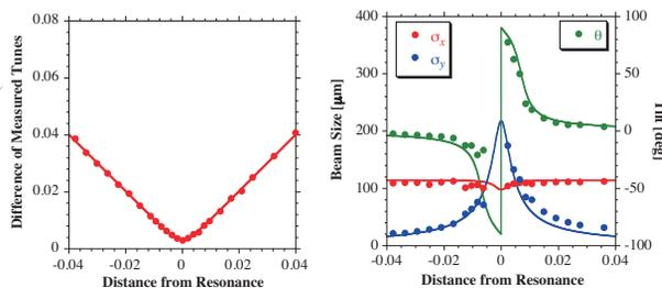
Figure 1: Tune survey at the SPring-8 storage ring.
