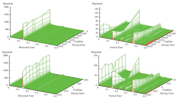
Figure 4: Fourier transform of beam oscillation in coupling correction.
