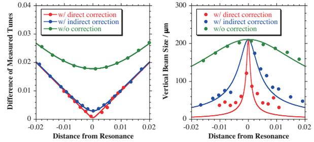
Figure 5: The tune differences and the vertical beam sizes near the linear coupling resonance for various coupling correction schemes.
