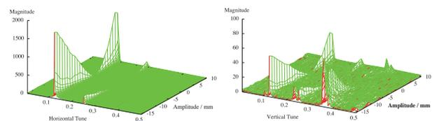
Figure 3: Fourier transform of horizontally kicked beam oscillation.
