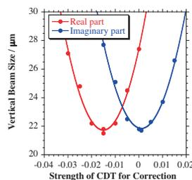
Figure 2: Coupling correction through vertical beam size.
