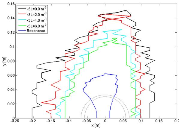
Figure 4: Dynamic aperture as a function of octupole and resonance strength. The chromaticity is corrected to satisfy the Hardt condition. For details refer to the text.
