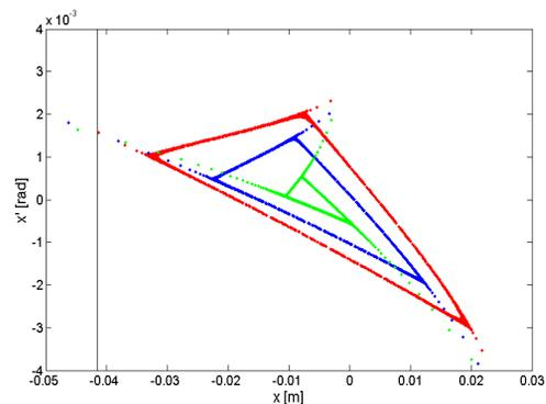
Figure 3: Separatrices of different sizes with identical spiral step and entrance angle at the septum.
