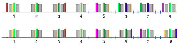
Figure 1: Location of sextupoles in the original (top) and the optimized (bottom) lattice. Resonance sextupoles, horizontal and vertical chromaticity sextupoles are colored red, blue, and pink, respectively. The green elements are orbit correctors, the yellow ones BPMs.
