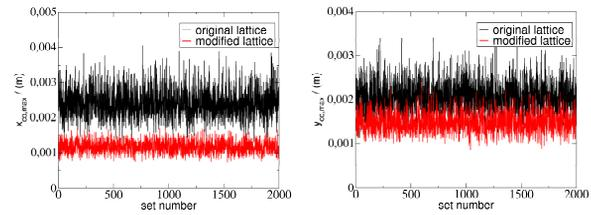
Figure 5: Residual orbit distortions in the horizontal and vertical plane for the original and the modified lattice.
