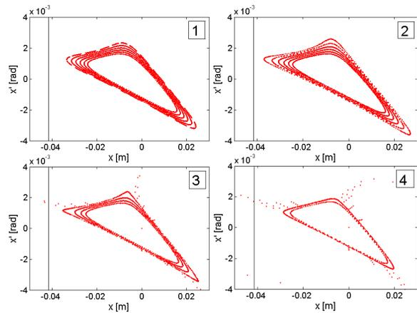
Figure 2: Trajectories in horizontal phase space as a function of octupole strength. The chromaticity is set to satisfy the Hardt condition. For details refer to the text.
