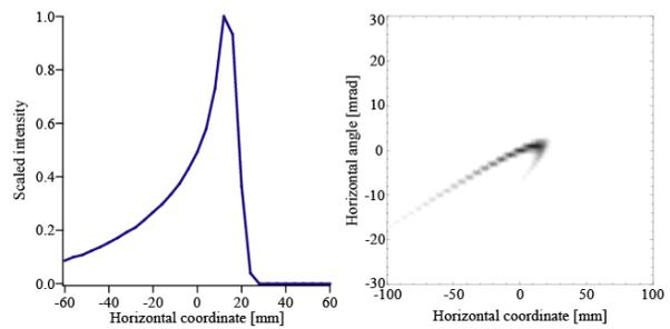
Figure 2: On-target real-space and phase-space distributions of the beam focused by a sextupole magnet, SXT1. The gradient of the sextupole magnet is set at  $19 \text{ m}^{-3}$ . The number of particles used in the simulation is  $10^6$ .
