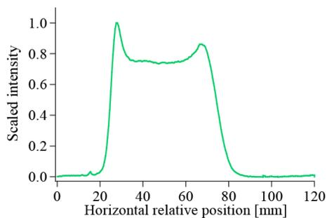
Figure 5: Horizontal relative intensity distributions of the proton beam measured using a radiochromic dosimetry film on the target [12]. The beam was focused by two sextupole magnets SXT1 and SXT2 with the field gradients of  $41 \text{ m}^{-3}$  and  $-54 \text{ m}^{-3}$ , respectively.
