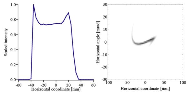
Figure 3: On-target real-space and phase-space distributions of the beam. The simulation parameters are the same as those in Fig. 2 except that another sextupole magnet SXT2 has been additionally turned on at the gradients of  $-52 \text{ m}^{-3}$ .
