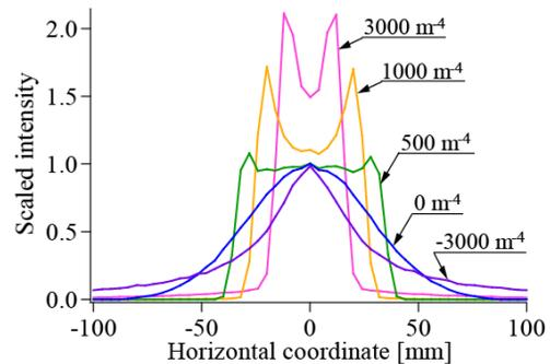
Figure 4: On-target real-space distributions of the beam focused by an octupole magnet, OCT1 with several different strengths.
