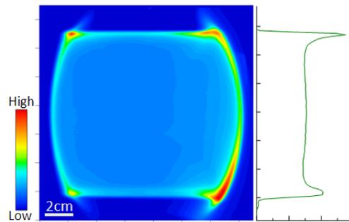
Figure 6: Spatial intensity distributions of the proton beam measured using a radiochromic film on the target. The beam was focused by two octupole magnets OCT1 and OCT2. The rms uniformity of the central 9-cm-square region is 5%.
