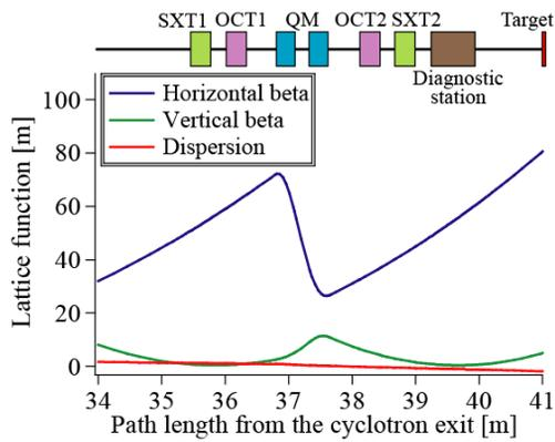
Figure 1: Schematic layout of magnets and the lattice functions around the end of the beam line at the JAEA AVF cyclotron. QM, SXT1 (SXT2), and OCT1 (OCT2) denote the quadrupole, sextupole, and octupole magnets, respectively. The axial length of the multipole magnets is 0.30 m. The beam-optical parameters have been adjusted so that the horizontal beta function is much larger than the vertical one at the multipole magnet locations for the reduction of the betatron coupling.
