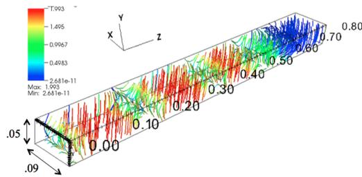
Figure 1: Wiggler field lines colored by field strength. The field is strongest in the y-direction
