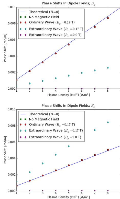
Figure 2: Phase shifts as a function of effective plasma density for uniform dipole magnetic fields. Top plot shows phase shifts for electric field polarized in the y-direction (lowest TE mode), and the bottom plot is for polarization in the x-direction (TE mode).
