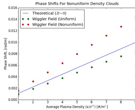
Figure 4: Phase shifts as a function of effective plasma density for modeled wiggler magnetic fields with two different plasma dielectric configurations. Simulated phase shifts are higher when the peak density is larger, although the average density is the same in both cases.
