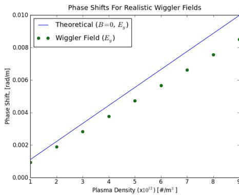
Figure 3: Phase shifts as a function of effective plasma density for modeled wiggler magnetic fields. Simulated phase shifts are about 20% lower than the nominal no magnetic field case at a density of  $9e^{12} e^-/m^3$ .
