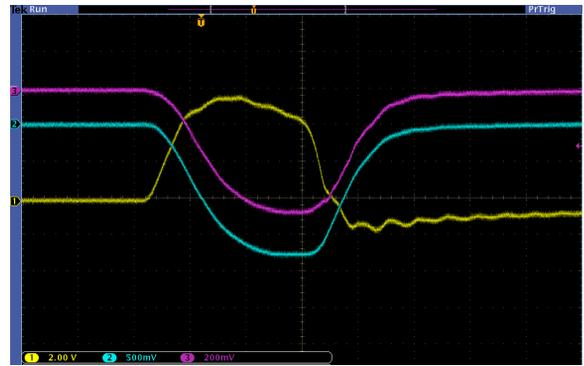
Figure 6: Typical 1  $\mu$ s 100 kV high voltage trace of modulator pulsing into low power resistive load. Yellow is a current transformer on the low voltage side of the transformer secondary that has saturated, Red is an accurate current transformer that has been installed on the high voltage end of the secondary, and Blue is an uncalibrated capacitive voltage divider.
