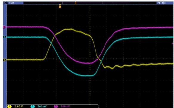
Figure 6: Typical 1  $\mu$ s 100 kV high voltage trace of modulator pulsing into low power resistive load. Yellow is a current transformer on the low voltage side of the transformer secondary that has saturated, Red is an accurate current transformer that has been installed on the high voltage end of the secondary, and Blue is an uncalibrated capacitive voltage divider.
