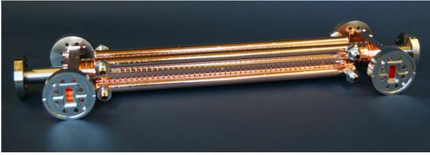
Figure 10: Completed T53 accelerator section.
