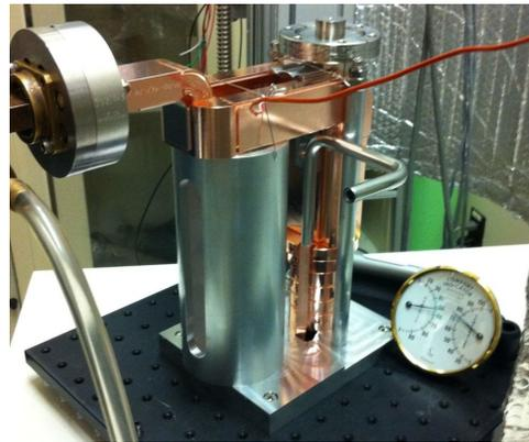
Figure 9: Cold test setup at SLAC for beadpull measurement and final tuning. RF gun currently under final bake.
