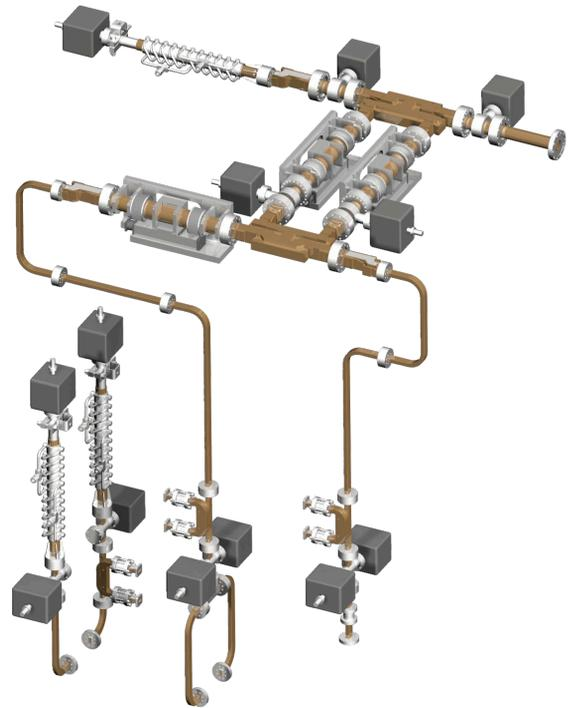
Figure 8: CAD rendering of test station RF distribution. Majority of components have been fabricated, delivered, and await installation.
