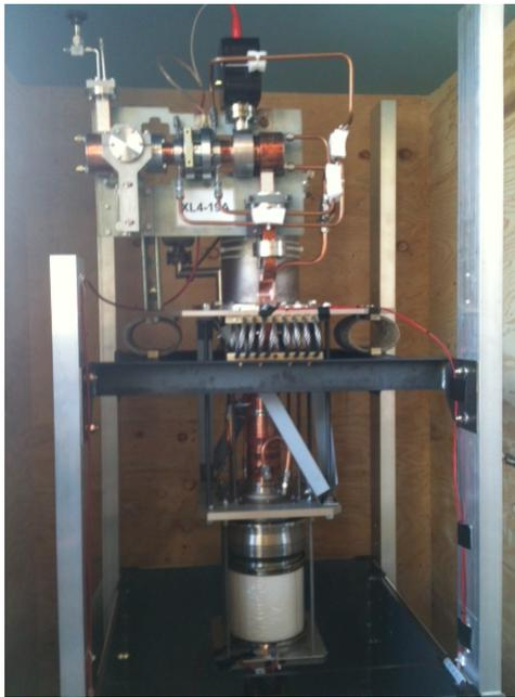
Figure 7: XL-4 klystron completed at SLAC and dressed for shipping.
