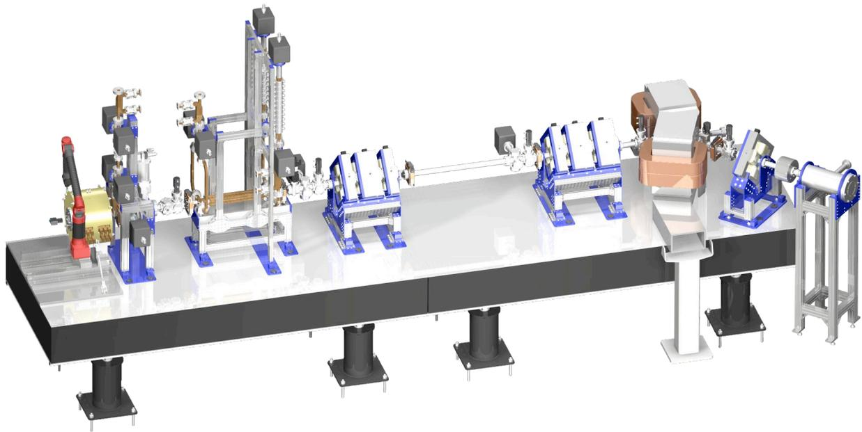
Figure 4: CAD rendering of the X-band test station.
