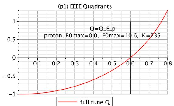
Figure 4:  $\beta$ -dependence of (magnetic) spin tune  $Q$  for protons in all-electric lattice. The spin is “globally frozen” for  $\beta=0.6$ . The spin is locally, but not globally, frozen for  $\beta=0.76$ , where  $Q$  is an integer other than zero.
