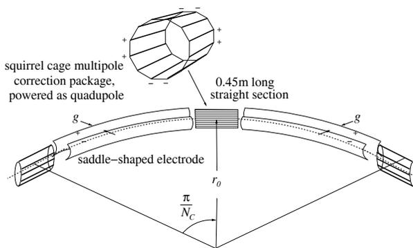
Figure 2: One cell of all-electric proton EDM lattice, with electrodes shaped for design field index  $m$ .
