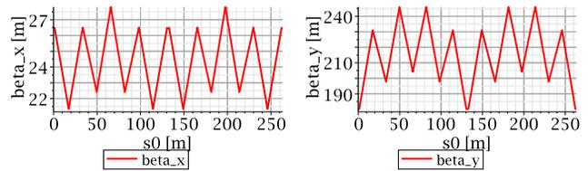
Figure 3: Plots of  $\beta$  functions of proton EDM lattice.  $\beta_y$  is necessarily very large, since  $Q_y$  has to be small.
