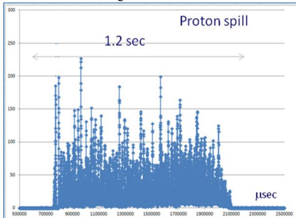
Figure 5: Time structure of a Proton beam spill.
