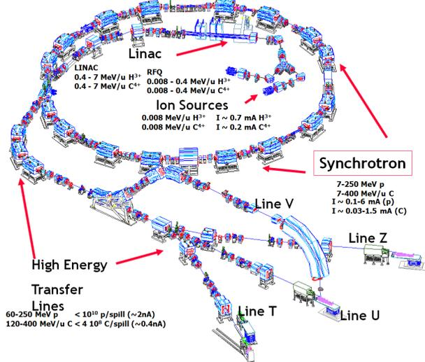
Figure 2: Layout of CNAO synchrotron and beam lines
