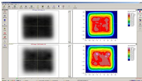
Figure 8: Homogenous square measured with a Proton beam.
