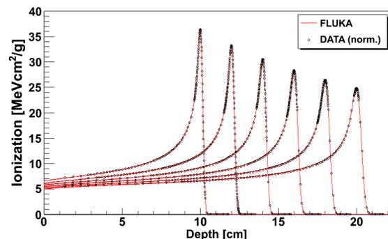
Figure 6: Proton Bragg peaks comparison between data and FLUKA simulations.
