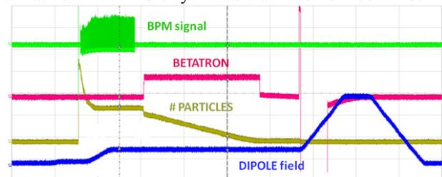
Figure 4: Machine cycle: a pick-up signal (green line), the Betatron ramp (pink line), the DCCT signal (yellow line) and synchrotron dipole field (blue line).
