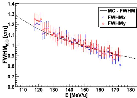
Figure 7: Beam dimensions in horizontal and vertical plane for a limited range of Proton beams.
