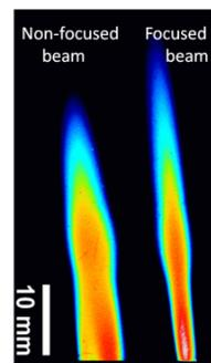
Figure 7: The divergence of non-focused beam and focused beam measured by the film.
