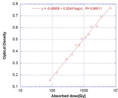
Figure 3: The calibration curve of HD-810 film.
