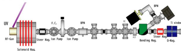
Figure 2: Schematic design of beamline.
