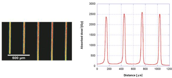
Figure 8: Left: The profile of multi-microbeam. Right: The spatial dose distribution (beam width:30µm, center-to-center distance:500µm ).
