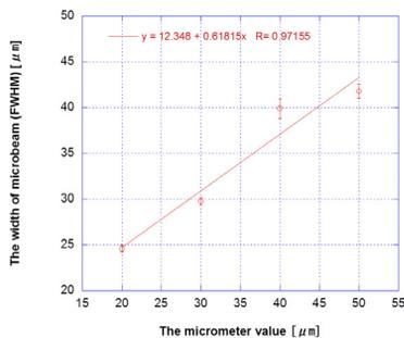
Figure 4: The slit width adjusted by the micrometer vs. microbeam width (FWHM) in the HD-810 film.
