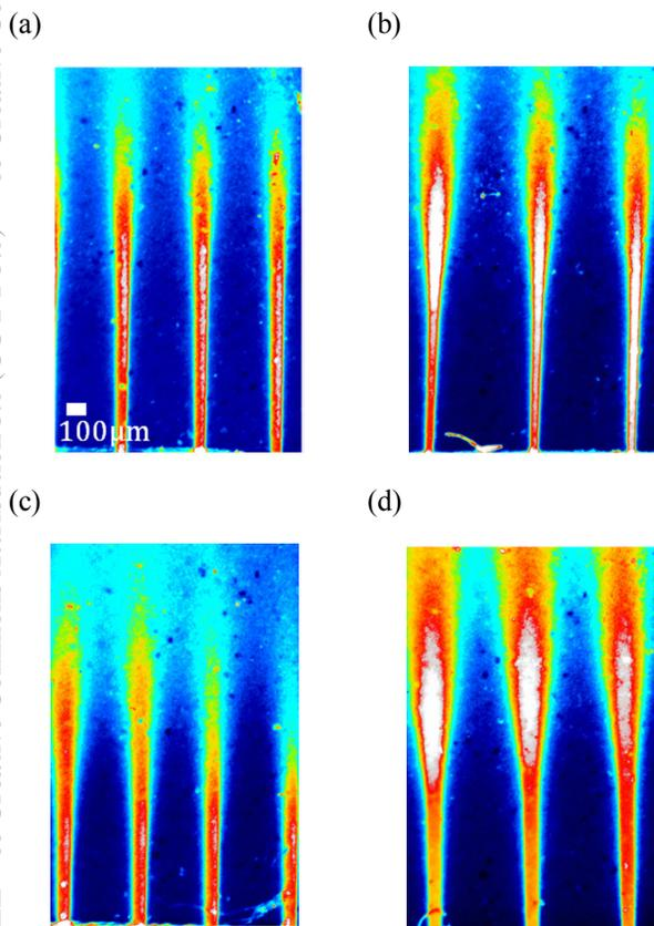
Figure 9: The microbeam distribution measured by films. (a) beam width: 20µm, distance: 400µm, (b) beam width: 20µm, distance: 500µm, (c) beam width: 30µm, distance: 400µm, (d) beam width: 30µm, distance: 500µm.
