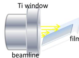
Figure 6: The schematic design of measuring the dose distribution using the HD-810 film.
