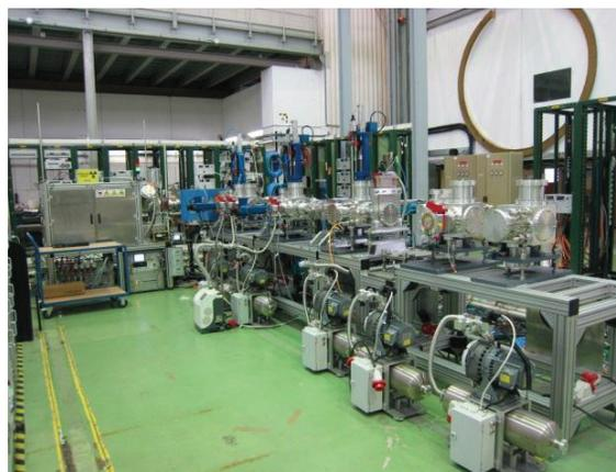
Figure 3: The MedAustron ITS at CERN, currently consisting of an ECR ion source, a spectrometer magnet and several different beam diagnostic tanks.
