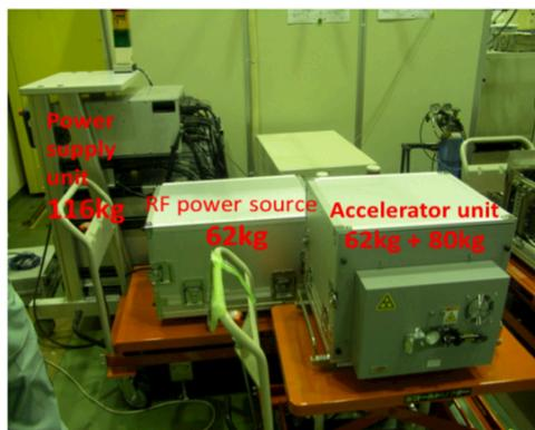
Figure 2: X-band 3.95MeV linac.
