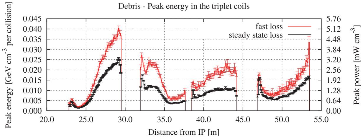
Figure 3: Longitudinal profile of peak( $\mathcal{E}$ ) and peak( $\mathcal{E}_{cable}$ ) along the coils of the magnets of the inner triplet, induced by the proton-proton collision debris. The red curve shows the energy density calculated for fast losses (fine mesh) and the black one for steady state losses at nominal luminosity (mesh corresponding to the cable size). The scale on the right axis applies only to the curve for steady-state.
