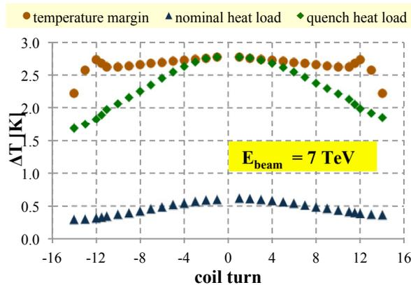
Figure 4: MQXB coil inner cable layer. The results of simulation for  $E_{\text{beam}} = 7 \text{ TeV}$  and  $L=10^{34} \text{ cm}^{-2} \text{ s}^{-1}$ .
