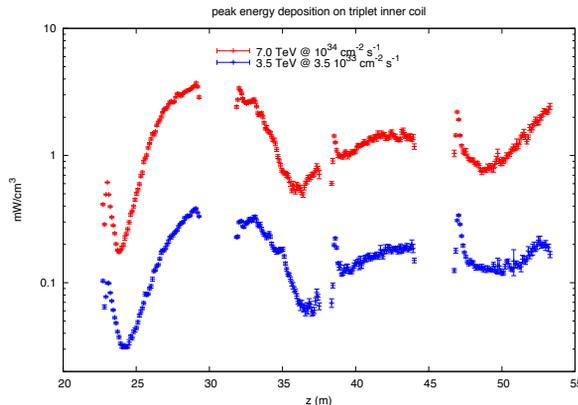
Figure 2: Longitudinal profile of  $\epsilon_{max}$  along the innermost coil layer of the magnets of the inner triplet, induced by proton-proton collision debris. Error bars indicate statistical uncertainties.
