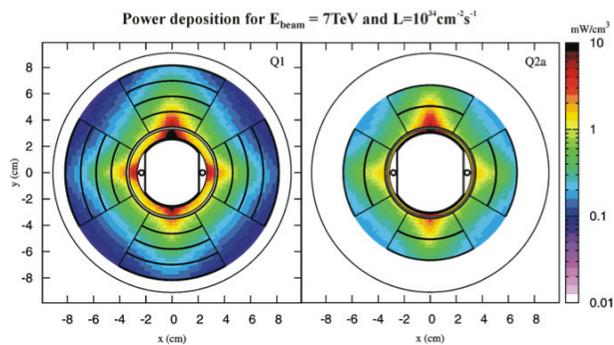
Figure 1: 2D map of the energy deposition in the Q1 (MQXA) and Q2A (MQXB) transverse section at the longitudinal position of the maximum, due to collision debris from proton-proton interactions. The geometrical model implemented in FLUKA is superimposed.
