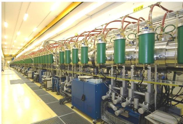
Figure 1: View of the 64 AIRIX induction accelerating cells. Each cell delivers 250 kV to the 2 kA electron beam.
