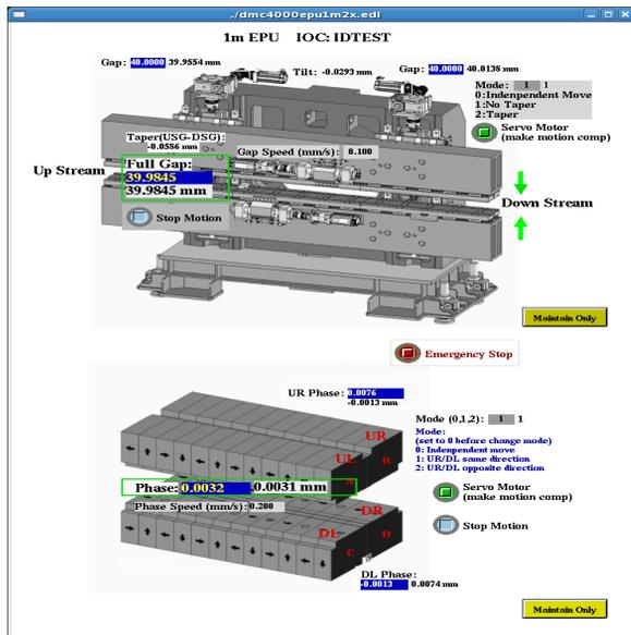
Figure 5: The preliminary GUI of the insertion devices.
