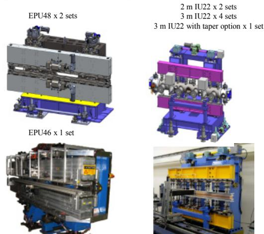
Figure 1: Insertion devices of TPS in the phase-I.
