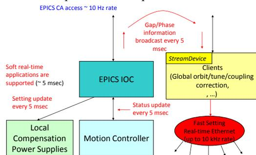
Figure 4: Local and global compensation schema for insertion device.
