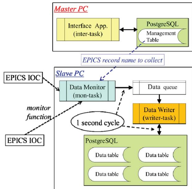
Figure 2: Software Configuration of DAC.
