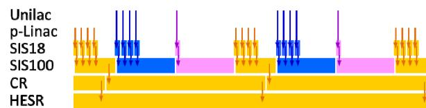
Figure 2: Periodic pattern and dependency of accelerators for parallel operation of anti-proton production (orange), RIB production (blue), and atomic physics (pink).
