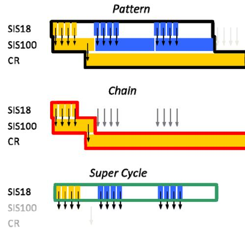
Figure 4: Pattern, chain, and super cycle, illustrated for the parallel operation of anti-proton production (orange) and RIB production (blue). The injector linacs as well as the HESR accumulating the anti-protons are omitted.
