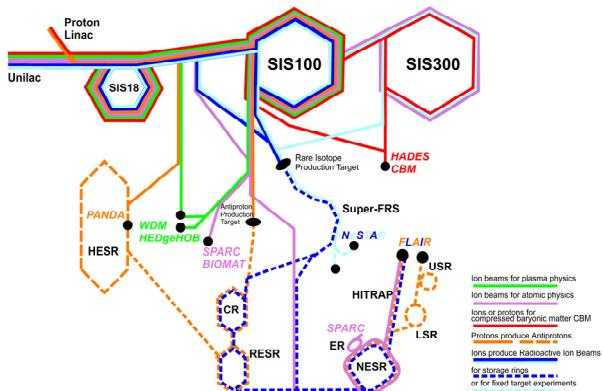
Figure 1: The accelerators and beamlines of the GSI/FAIR accelerator complex.
