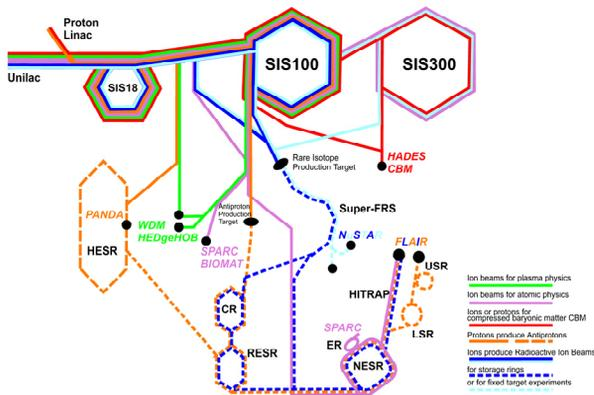
Figure 1: The accelerators and beamlines of the GSI/FAIR accelerator complex.
