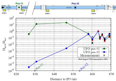
Figure 5: Comparison of measured and simulated BLM dose patterns corresponding to UFO-induced beam losses in the standard arc cell 19R3. Simulations were performed for two potential UFO locations (*Pos #1*, *Pos #2*). The signal at the six standard quadrupole BLMs (860 m - 870 m) and the additional diagnostics BLMs (820 m - 860 m) normalized to the highest signal in the quadrupole BLMs is shown (courtesy of A. Lechner and the FLUKA team [8]).
