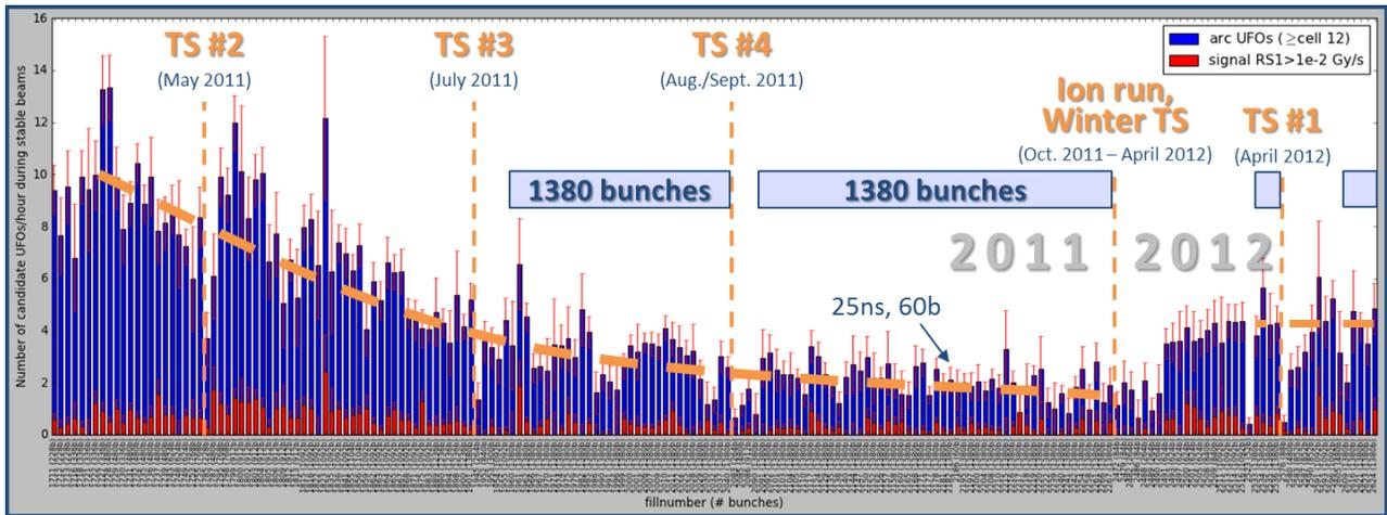
Figure 2: The rate of 5957 arc UFO events ( $\geq$  cell 12) during stable beam operation at top energy (stable beams) for all proton fills with at least one hour of stable beams between April 2011 and May 2012. During 2011, the rate decreased from about 10 events per hour to about 2 events per hour. The rate is reduced during the low intensity fills directly after the technical stops (TS).
