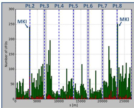
Figure 3: The spatial distribution of 7784 UFO events at 3.5 TeV between April and October 2011. The red bars correspond to events with a peak loss  $> 10^{-2}$  Gy/s. The vertical dashed blue lines indicate the locations of the insertion regions. Gray areas are excluded from UFO detection.
