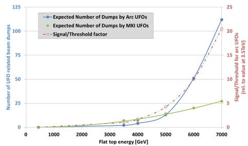
Figure 6: The expected number of beam dumps by arc UFOs and MKI UFOs and the expected scaling of BLM signal/BLM threshold for different energies. All 2011 UFO events since 14<sup>th</sup> April are considered (based on [8, 6, 9]).
