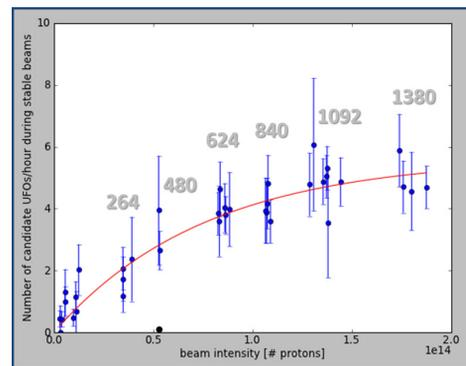
Figure 4: The rate of 500 arc UFO events ( $\geq$  cell 12) as a function of the maximum beam intensity of the fills during the fast intensity ramp up in the beginning of 2012. The gray numbers indicate the number of bunches.
