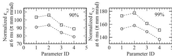
Figure 7: Horizontal (circle) and vertical (square) normalized emittances obtained at 6 ms in Fig. 6, plotted as a function of the painting parameter ID in Table 1.
