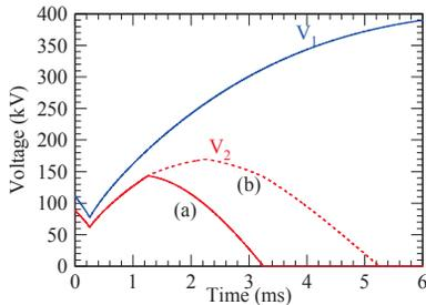
Figure 3: Second harmonic rf voltage patterns with different durations (a) and (b) used for longitudinal painting in the present work.
