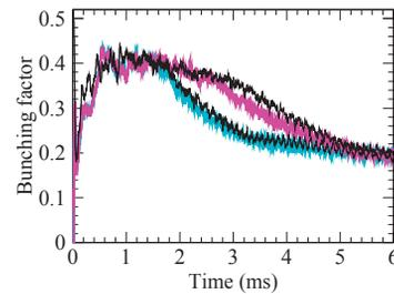
Figure 5: Bunching factor for the first 6 ms measured for the painting parameter IDs 2 (light blue) and 3 (pink) in Table 1, where the corresponding numerical simulation results are plotted by black curves.
