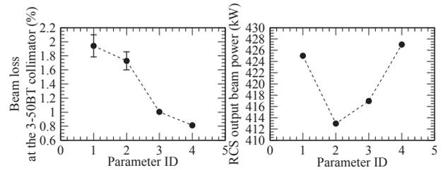
Figure 4: [Left] Painting parameter dependence of the beam loss at the 3-50BT collimator measured for the extracted beam from the RCS, where the horizontal axis corresponds to the painting parameter IDs in Table 1. [Right] Similar dependence of the RCS output intensity measured upstream of the 3-50BT collimator in parallel with the above beam loss measurement.
