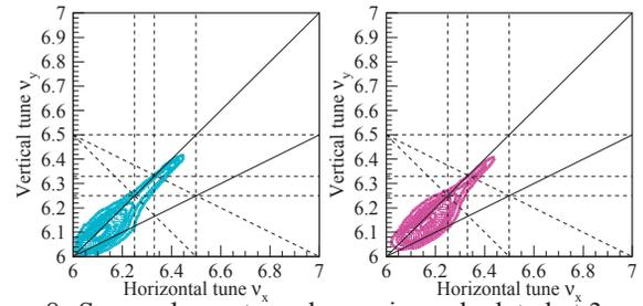
Figure 8: Space-charge tune depression calculated at 3 ms for the parameter IDs 2 (left) and 3 (right) in Table 1, where the bare tunes are set at (6.45, 6.42).
