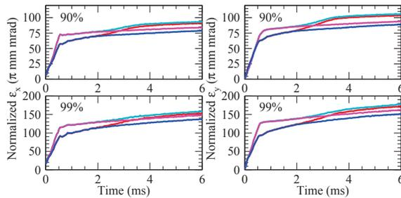
Figure 6: Time evolution of the horizontal (left) and vertical (right) normalized emittances calculated for the first 6 ms with the parameter IDs 1 (red), 2 (light blue), 3 (pink) and 4 (blue) in Table 1, where different emittances encircling 90 and 99% of the macro-particles are plotted for each parameter ID.
