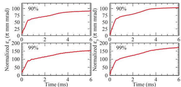
Figure 1: Time evolution of the horizontal (left) and vertical (right) normalized emittances calculated for the first 6 ms, where different emittances encircling 90 and 99% of the macro-particles are plotted.
