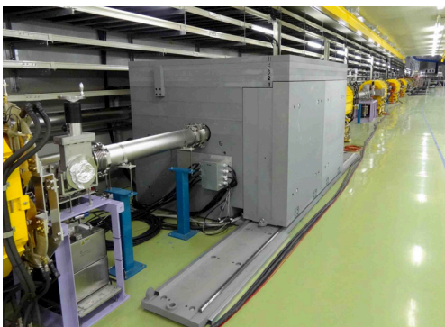
Figure 4: New collimator system installed in the SX straight section.
