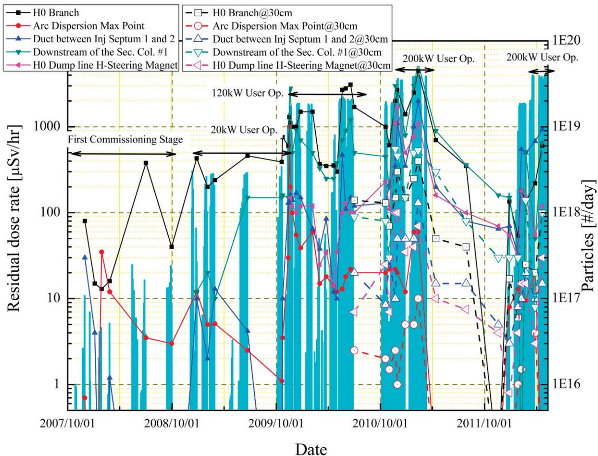
Figure 3: the history of the residual dose of typical loss point and output power of RCS.
