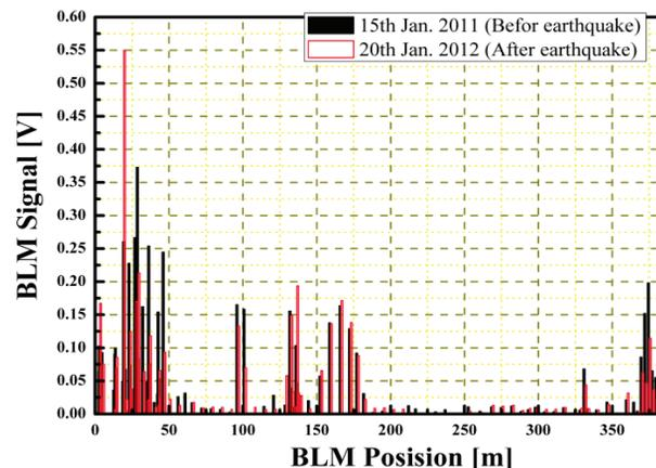
Figure 1: BLM signals at 300 kW output power operations before and after the earthquake.
