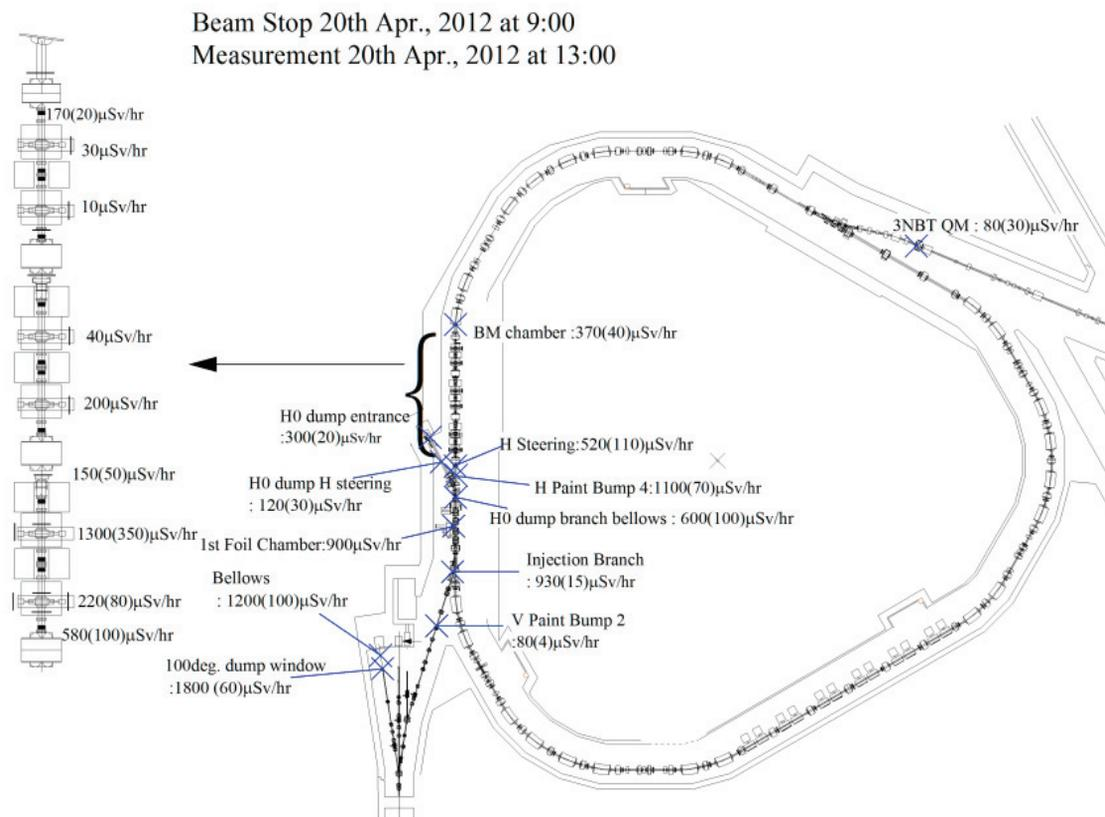
Figure 2: Residual dose distribution with 200kW operation after the earthquake.
