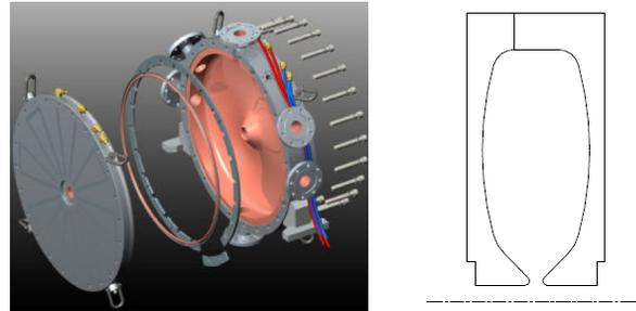
Figure 2: The JPAW elliptical cavity, courtesy of Jim Potter, Conceptual Design Report FE-EE-019.
