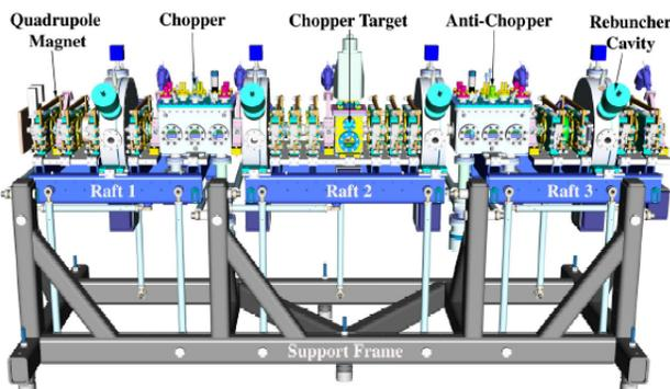
Figure 1: A layout of SNS MEBT, courtesy of D. Oshatz et al, PAC 2001.
