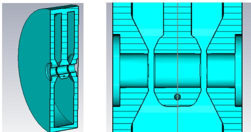
Figure 3: The DTL type cavity with double-gaps.
