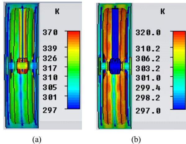
Figure 5: Temperature distribution of two gap cavity with SS304 cavity wall – (a) SS 304 tube and stem (b) Copper tube and stem.
