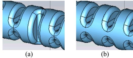
Figure 1: (a) Interleaved (b) Non-interleaved RA cavity.
