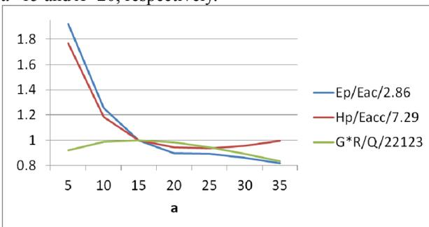
Figure 5:  $H_{pk}/E_{acc}$  and  $E_{pk}/E_{acc}$  w.r.t.  $a$  ( $r=35$ ,  $A=20$ ).
