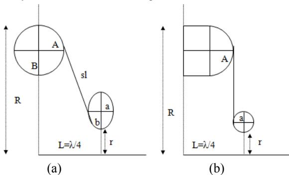
Figure 4: Cavity shape parameters : (a) TESLA (b) RA.
