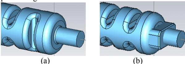
Figure 9: (a) Cylindrical (b) Rectangular End-Cell pipe.
