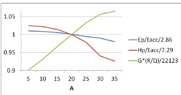
Figure 6:  $H_{pk}/E_{acc}$  and  $E_{pk}/E_{acc}$  w.r.t.  $A$  ( $r=35$ ,  $a=15$ ).
