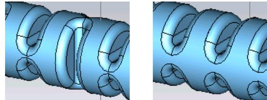
Figure 1: (a) Interleaved (b) Non-interleaved RA cavity.
