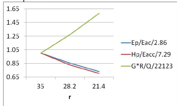
Figure 7:  $H_{pk}/E_{acc}$  and  $E_{pk}/E_{acc}$  w.r.t.  $r$  ( $a=15$ ,  $A=20$ ).
