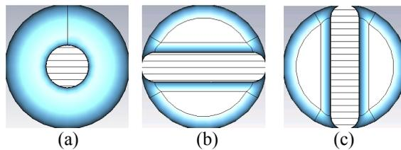
Figure 2: Section view of TESLA and RA cavity (a) TESLA (b) RA – π phase (c) RA – π + π/2 phase.
