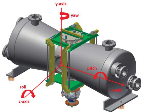
Figure 1: (Top) The cavity alignment coordinate system and slow tuner. Notice the small circular pucks on the bottom of the cavity (two visible) these are the kinematic supports. (Bottom) Slow tuner assembly. The slow tuner bellows actuator is on the left and the outward force on the wire ropes is translated into a reduction of the beam-line length of the cavity by the bars that attached to the beam port in the middle and the wire ropes on their ends.
