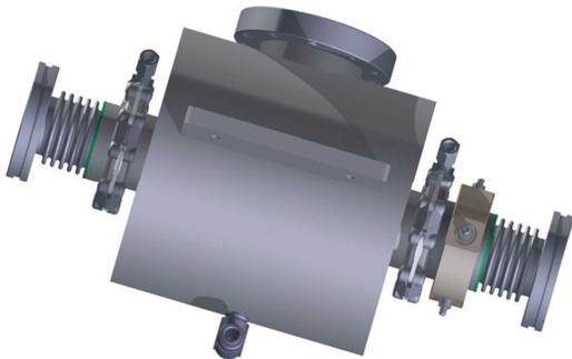
Figure 2: The superconducting magnet with EVAC CeFiX flanges, formed metal bellows which connect to the half-wave resonators and the beam-position-monitor. The magnet integrates an 6 T superconducting solenoid with x-y steering coils. As shown the length is 40 cm.
