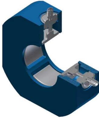
Figure 3: A quarter-section view of the BPM. As shown the BPM is 1" long with a maximum diameter of 3.7" and a beam aperture of 33 mm, the PXIE requirement.
