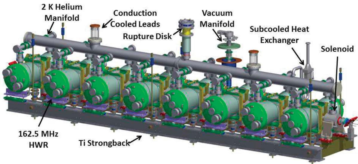
Figure 4: The cryomodule beam-line assembly. The clean cavity vacuum manifold is behind the assembly but the lid penetration is visible behind the helium manifold. The assembly as shown is 5.9 meters long. The cryomodule still remains to be designed but initial estimates give a width and a height of 1.7 m and 2.0 m respectively.
