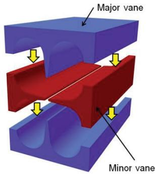
Figure 3: Simplified exploded view of one RFQ section.
