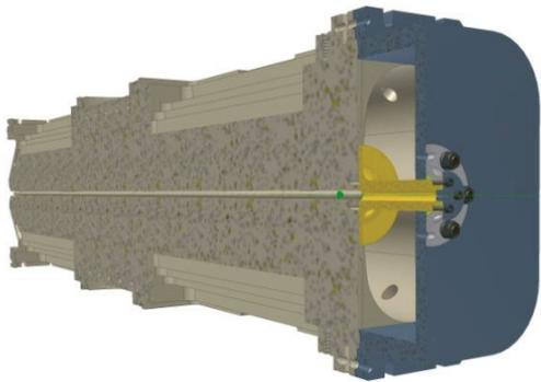
Figure 4: Section view of bead-pull / RF test end flange.
