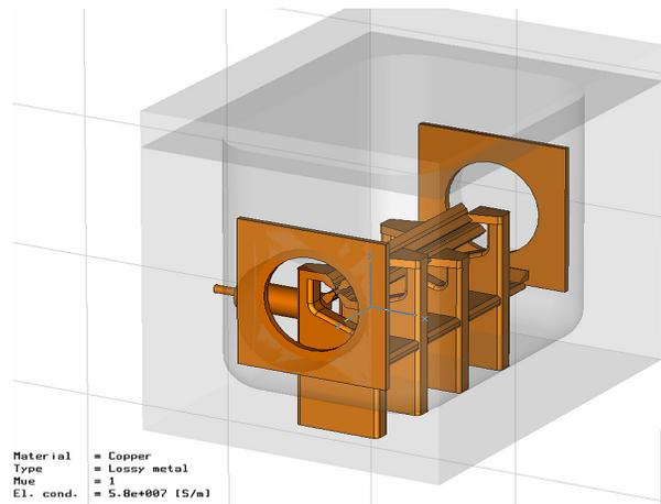
Figure 6: A new cw RFQ Prototype (175 MHz).
