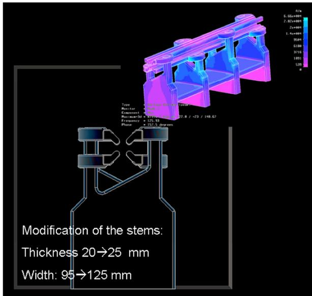
Figure 5: Modification of the stems.
