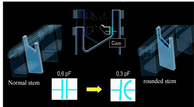
Figure 4: The capacity between stems and electrodes.
