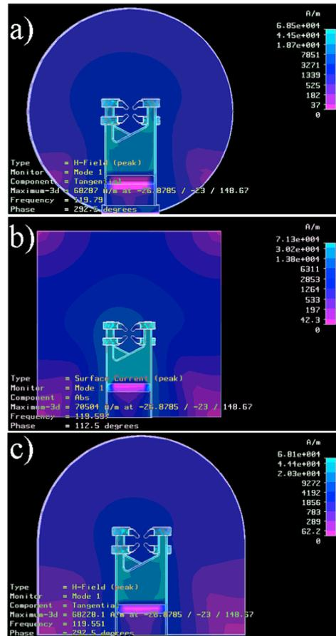
Figure 3: The magnetic field (ABS) inside the tank.
