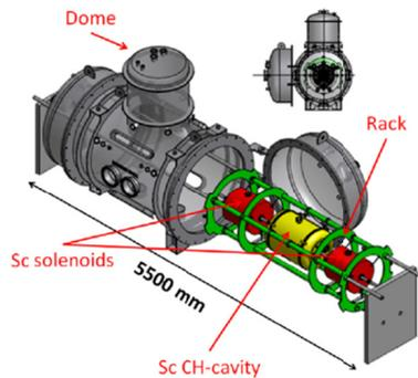
Figure 5: The demonstrator cryomodule for the new sc-w-linac at GSI.
