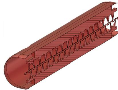
Figure 4: Simulation model of the first HE-linac IH-cavity.
