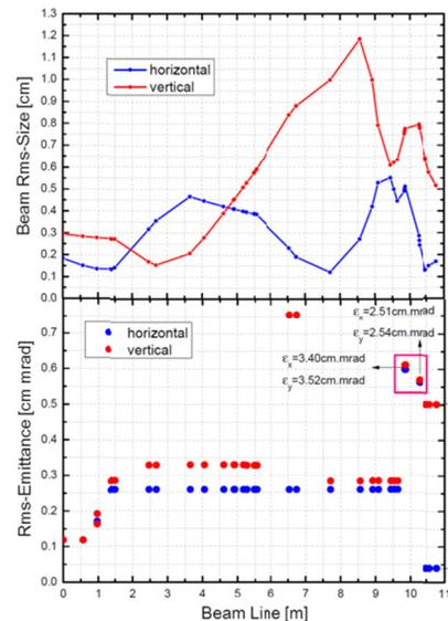
Figure 7: Beam envelopes and rms-emittances along the emittance-transfer beamline.
