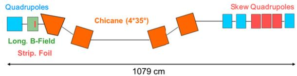
Figure 6: Beam line to transfer emittance from the horizontal to the vertical plane.
