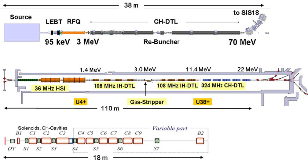
Figure 2: Conceptual layouts of the future linacs at GSI. From top to bottom: proton linac, sc cw-linac, and high energy linac. Dimensions are not to scale.
