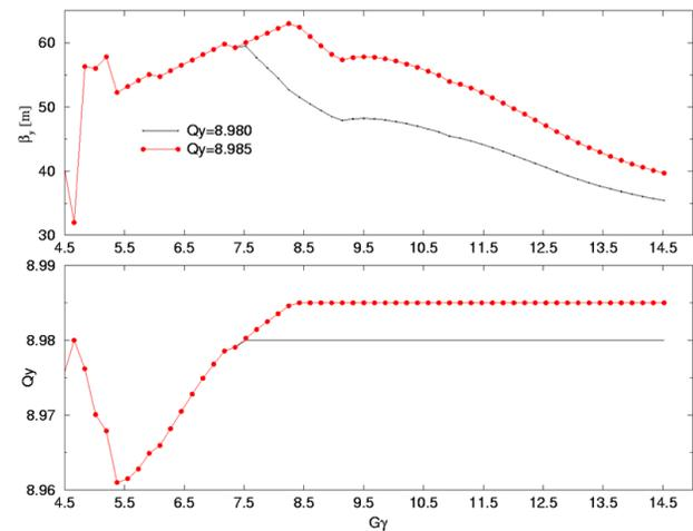
Figure 5: The beta function ( $\beta_y$ ) (top), and the vertical tune  $Q_y$  (bottom) as a function of  $G\gamma$ . The red line corresponds to the AGS optics where we constrain the  $Q_y$  tunes to have the value of 8.985 for values of  $G\gamma > 7.5$ , and the black line corresponds to the AGS optics where we constrain the  $Q_y$  tunes to have the value of 8.980 for values of  $G\gamma > 7.5$ .
