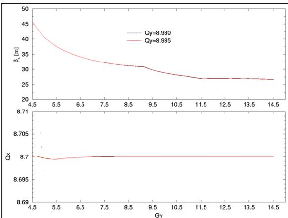
Figure 4: The beta function ( $\beta_x$ ) (top), and the horizontal tune  $Q_x$  (bottom) as a function of  $G\gamma$ .
