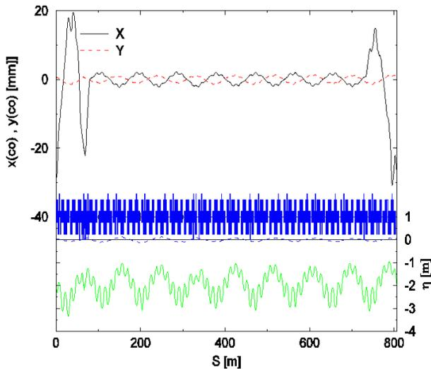
Figure 3: The Horizontal ( $X_{cod}$  lack solid line), and the vertical ( $Y_{cod}$  red dashed line) closed orbit displacements, at beam injection in AGS. The  $X_{cod}$ , is generated by the excitation of the "L20 Bump", and the "Cold helix A20 Bump" (see text). The linear coupling introduced by the helices generates the nonzero value of the  $Y_{cod}$ .
