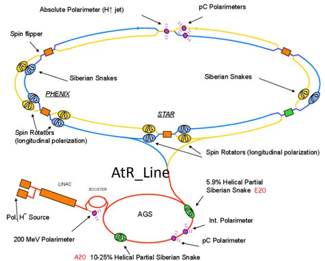
Figure 1: The RHIC Complex with the location of the A20 and E20 partial helices of the AGS.
