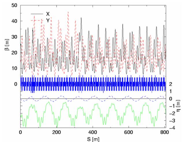
Figure 2: The beta ( $\beta_{x,y}$ ) functions, and the dispersion functions ( $\eta_{x,y}$ ) at injection energy ( $G\gamma = 4.5$ ) plotted along the AGS. The vertical dispersion function (blue dashed line) is due to the coupling of the partial helices.
